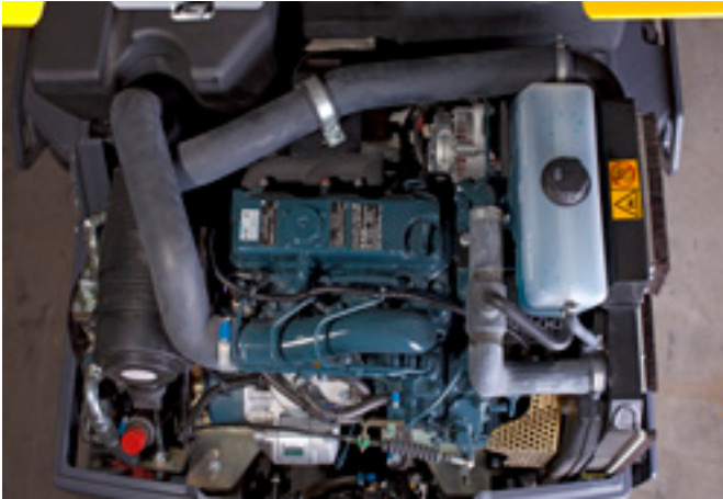
Silent and powerful water-cooled Kubota diesel engine. The large easy-to-open engine hood contributes to great accessibility.
