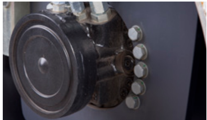
Fail-safe brakes on both drums (or drum + combi wheels), which apply automatically in the event of a failure in the engine, hydraulics or an electrical fault in the brake system.
