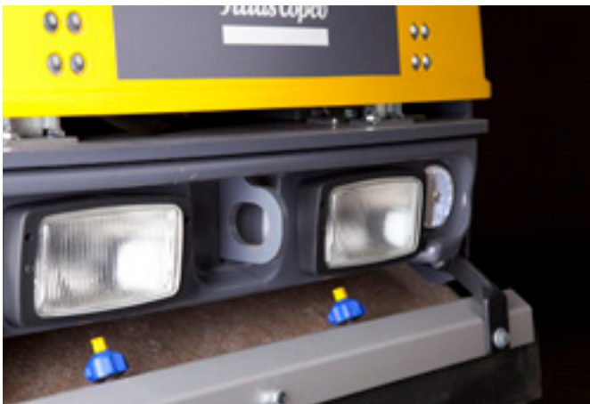
Pressurized sprinker system with a powerful water pump and self-draining sprinker tubes and nozzles.
